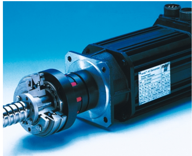
EAS ® -NC Lastic Backlash-free version in a directly driven servo axis. This combination limits the torque precisely to the pre-set value, compensates for shaft misalignments and damps critical vibrations.
